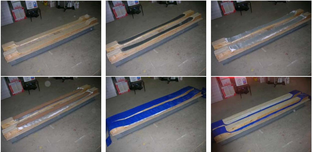
*Figure 2.1.2 – Press and mold layup process. From top left: empty mold, then the black p-tex base is added, then successive layers, until the bladder and top mold are placed. Bottom right: the all parts of the press are put into place, and the pressure is raised in the bladder hoses, evenly distributing the pressure along the ski.*
