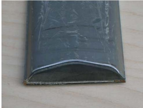
*Figure 1.2.3 – Example of Monocoque construction with a foam core*
