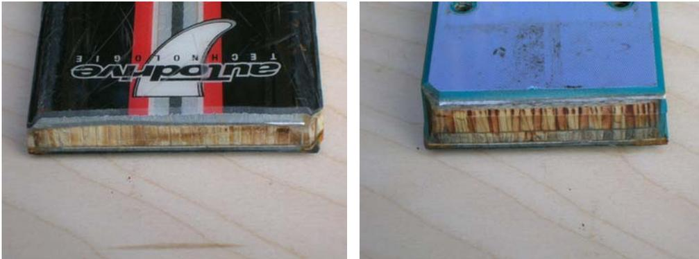
*Figure 1.2.1 – Examples of Sandwich construction*
