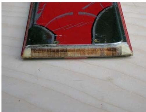
*Figure 1.2.4 – Example of cap-sandwich hybrid construction*
