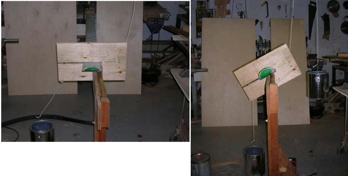
*Figure 3.2.1 Torsional Stiffness test. The right weight is hung on a sliding pulley, assuring the force applied is perfectly vertical.*
