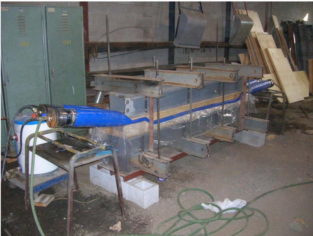
*Fig. 0.0.1 The homemade ski press*
